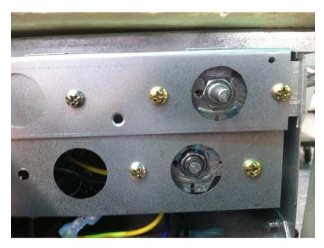
18) If the model # ends in any letter other than "D" and has a white plastic cam timer use the opening to the left to mount the cube size control (see below)
